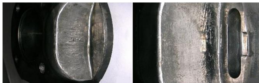
Fig. 4 Contact area of the moving core and the shaped part of the mold - mechanical wear
