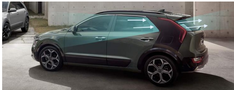
Figure 6. Production version of the integrated air duct in the vehicle's C-pillar Kia Niro MY 2022 [11].
