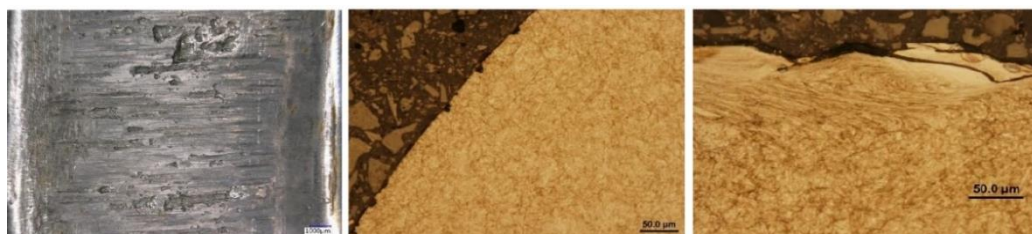
Fig. 5 Area of repeated contact - impact of the movable core parallel to the parting plane with the surface of the mold part – inserts
