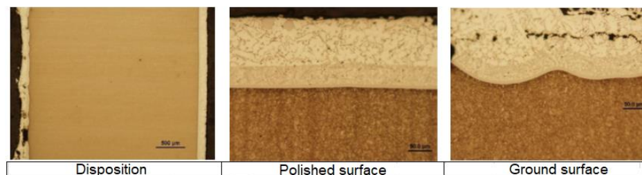
Fig. 2 Interface of insert material and AlSi8Cu3 after 15 minutes exposure in the melt at 680 \pm 20 °C
