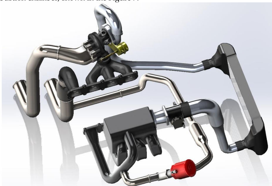
Figure 7. Technical solution of intake air and recirculation of already burned gases.
