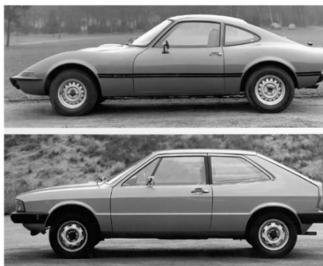
Figure 2. Comparison of two cars with the same air coefficient and different body shape. From above Opel GT MY 1968 c_d = 0,41 , A = 1,51 \text{ m}^2 , from below VW Scirocco MY 1974 c_d = 0,41 , A = 1,73 \text{ m}^2 [1].
